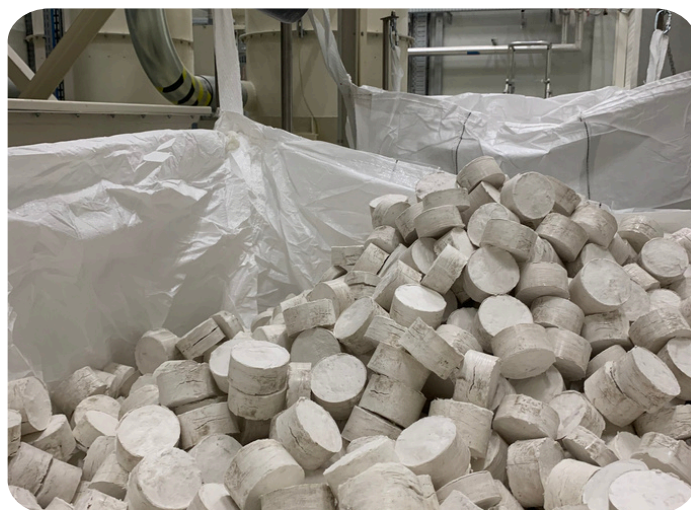
Photo of cellulose briquettes generated by waste fibers at the Gdansk Plant.
